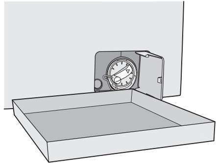
5. Pull out the emergency emptying cap from the filter cover, using pliers.
